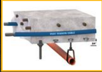
Post Tension Concrete
