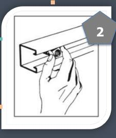
A 90-degree clockwise turn aligns the grooves in the nut with the inturned edges of the channel.
