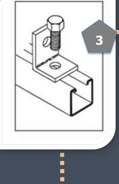
Next, bolt the additional channel section in place by following the procedures outlined in steps 1-3.
