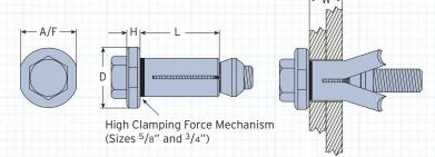
Sizes 5/8" & 3/4", known as the Hollo-Bolt HCF, feature a patented High Clamping Force mechanism to produce up to three times more clamping force than the same sized product without the mechanism. The significance of clamping force and the superior performance of Lindapter's unique Hollo-Bolt HCF is illustrated on page 7 of the Hollo-Bolt brochure, which can be downloaded at www.hollo-bolt.com
