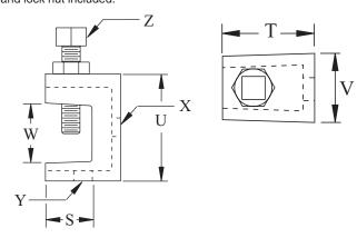
et Screw Torque = 3 Ft-Lb eck Nut Torque = 3.5 Ft-Lb
