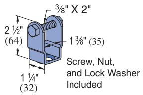
Clevis hanger to be used with P2676 or P2682 to provide angle adjustment and 15° (0.08  $\varpi$ ) free swing for up to ½" (13) rod suspension. Order swivel nuts P2679-4, -6, or -8 as required.
