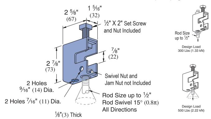
Clamp P2676 provides a means of rod suspension where a free swing of up to  $15^{\circ}$  (0.8 $\varpi$ ) is required. Clamp will accommodate  $\frac{1}{4}$ " (6),  $\frac{3}{6}$ " (10), or  $\frac{1}{2}$ " (13) rods. Order swivel nuts P2679-4,-6, or -8 as required. Clamp may also be used with P2677 as illustrated in application drawings.
