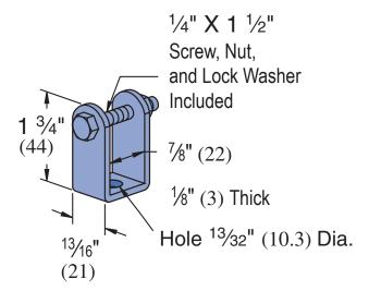
Clevis hanger to be used with P2675 to provide angle adjustment for up to %" rod suspension as illustrated.
