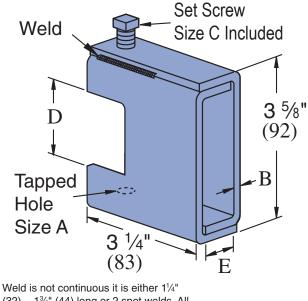
(32) -  $1\frac{3}{4}$ " (44) long or 2 spot welds. All welds are on the top and bottom.
