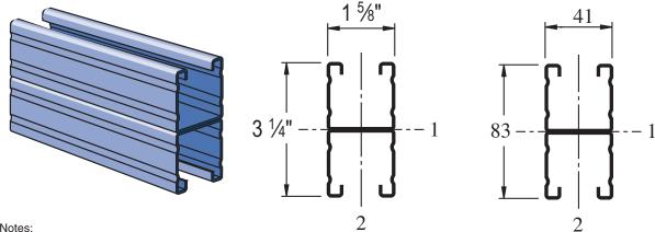
Wt/100 Ft: 232 Lbs (346 kg/100 m) Allowable Moment 9,570 In-Lbs (1,080 N•m) 16 Gauge Nominal Thickness .060" (1.5mm)
