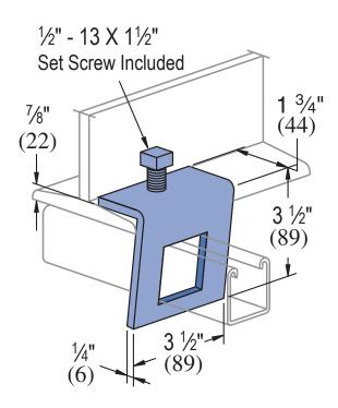
Design Load Each 500 Lbs (2.22 kN) Use in Pairs Only
