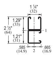
Wt/100 Ft: 207 Lbs (308 kg/100m) Allowable Moment 6,760 In-Lbs (760 N•m) 14 Gauge Nominal Thickness .075" (1.9mm)
