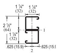
Wt/100 Ft: 207 Lbs (308 kg/100m) Allowable Moment 7,930 In-Lbs (900 N•m) 14 Gauge Nominal Thickness .075" (1.9mm)
