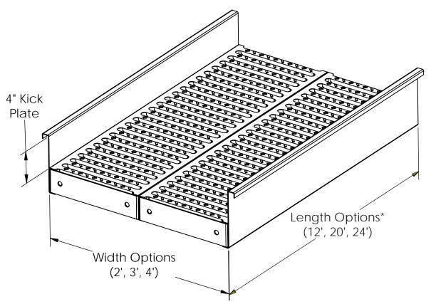
\* These lengths are for a single platform assembly. Longer lengths can be accomplished by splicing platforms together.
