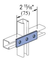
Standard Dimensions for 13/16" (21mm) width series channel fittings (Unless Otherwise Shown on Drawing)
