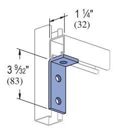
Standard Dimensions for 1<sup>1</sup>/4" (32 mm) width series channel fittings (Unless Otherwise Shown on Drawing) Hole Diameter: <sup>13</sup>/<sub>20</sub>" (10mm); Hole Spacing - From End: <sup>5</sup>/<sub>8</sub>" (16 mm); Hole Spacing - On Center: <sup>1</sup>/<sub>8</sub>" (38= mm); Width: <sup>1</sup>/<sub>4</sub>" (32mm); Thickness: <sup>3</sup>/<sub>6</sub>" (5mm)
