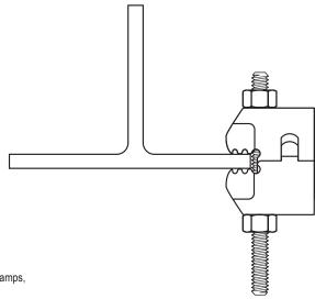
Designed to significantly reduce installation time, while offering greater performance than cast beam clamps,
