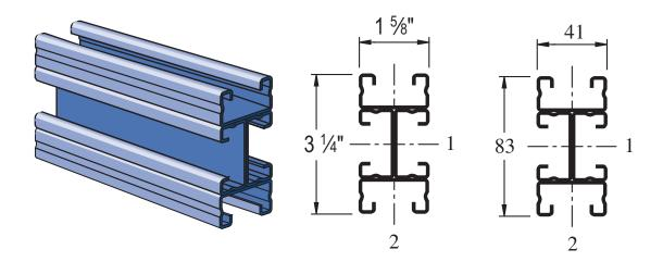
Wt/100 Ft: 331 Lbs (493 kg/100 m) Allowable Moment 13,650 In-Lbs (1,540 N•m) 16 Gauge Nominal Thickness .060" (1.5mm)
