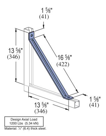
Standard Dimensions for 15/8" (41mm) width series channel fittings (Unless Otherwise Shown on Drawing)
