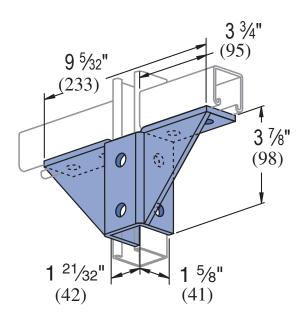
Standard Dimensions for 15/8" (41mm) width series channel fittings (Unless Otherwise Shown on Drawing)
