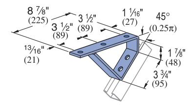
Standard Dimensions for 15/8" (41mm) width series channel fittings (Unless Otherwise Shown on Drawing)
