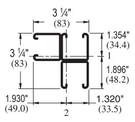
Wt/100 Ft: 566 Lbs (843 kg/100 m) Allowable Moment 18,680 In-Lbs (2,110 N•m) 12 Gauge Nominal Thickness .105" (2.7mm)
