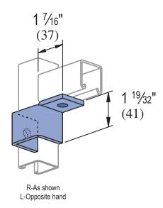
Standard Dimensions for 11/4" (32 mm) width series channel fittings (Unless Otherwise Shown on Drawing)
