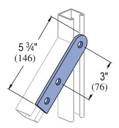
Standard Dimensions for 11/4" (32 mm) width series channel fittings (Unless Otherwise Shown on Drawing)
