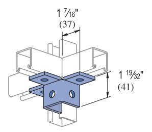
Standard Dimensions for 11/4" (32 mm) width series channel fittings (Unless Otherwise Shown on Drawing)
