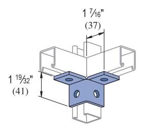
Standard Dimensions for 11/4" (32 mm) width series channel fittings (Unless Otherwise Shown on Drawing)
