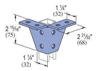
Standard Dimensions for 11/4" (32 mm) width series channel fittings (Unless Otherwise Shown on Drawing)
