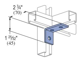
Standard Dimensions for 1<sup>1</sup>/<sub>4</sub>" (32 mm) width series channel fittings (Unless Otherwise Shown on Drawing) Hole Diameter: <sup>13</sup>/<sub>2</sub>" (10mm); Hole Spacing - From End: <sup>5</sup>/<sub>8</sub>" (16 mm); Hole Spacing - On Center: <sup>11</sup>/<sub>2</sub>" (38= mm); Width: <sup>11</sup>/<sub>4</sub>"(32mm); Thickness: <sup>3</sup>/<sub>6</sub>" (5mm)
