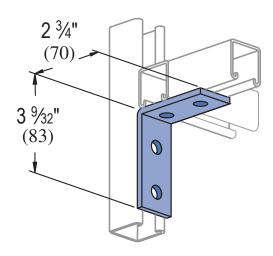
Standard Dimensions for 11/4" (32 mm) width series channel fittings (Unless Otherwise Shown on Drawing)
