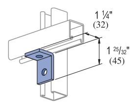
Standard Dimensions for 11/4" (32 mm) width series channel fittings (Unless Otherwise Shown on Drawing)
