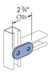
Standard Dimensions for 1<sup>1</sup>/<sub>4</sub>" (32 mm) width series channel fittings (Unless Otherwise Shown on Drawing) Hole Diameter: <sup>13</sup>/<sub>2</sub>" (10mm); Hole Spacing - From End: <sup>5</sup>/<sub>8</sub>" (16 mm); Hole Spacing - On Center: 1<sup>1</sup>/<sub>2</sub>" (38= mm); Width: 1<sup>1</sup>/<sub>4</sub>"(32mm); Thickness: <sup>3</sup>/<sub>6</sub>" (5mm)
