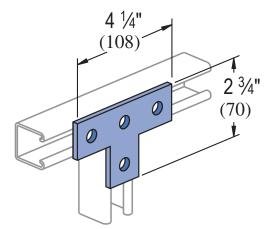
Standard Dimensions for 1<sup>1</sup>/4" (32 mm) width series channel fittings (Unless Otherwise Shown on Drawing) Hole Diameter: <sup>13</sup>/<sub>2</sub>" (10mm); Hole Spacing - From End: <sup>5</sup>/<sub>4</sub>" (16 mm); Hole Spacing - On Center: <sup>11</sup>/<sub>2</sub>" (38= mm); Width: <sup>11</sup>/<sub>4</sub>"(32mm); Thickness: <sup>3</sup>/<sub>6</sub>" (5mm)
