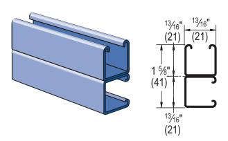
Wt/100 Ft: 73 Lbs (108 kg/100 m) Allowable Moment 1,550 ln-Lbs (180 N•m) 19 Gauge Nominal Thickness .040" (1.0 mm)
