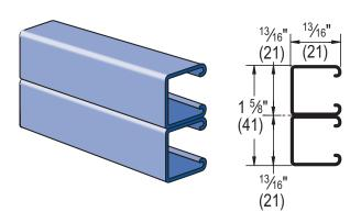
Wt/100 Ft: 73 Lbs (108 kg/100 m) Allowable Moment 1,820 ln-Lbs (210 N•m) 19 Gauge Nominal Thickness .040" (1.0 mm)
