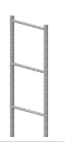
Climb ladder using a recognised safe method of climbing for first man up - i.e. twin lanyard system to give continuous attachment.
