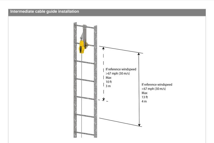
Descend the ladder to the position of the first helix cable guide, dependent upon site reference wind speed for external installations. Depending upon the location of the ladder and local weather patterns, irregular spacing of the cable guides will reduce cable deflection resulting from wind buffeting.
