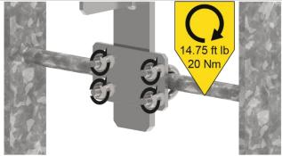
Evenly tighten the nuts with the deep socket to a torque of 14.75 ft lb (20 Nm).
