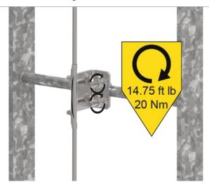
Evenly tighten the nuts using the deep socket to a torque of 14.75 ft lb (20 Nm).
