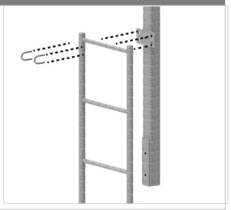
Locate the extension post top anchor at the centre of the top three rungs as shown. Insert the supplied Ubolts over the top ladder rung and through the slots of the extension post clamping bracket.
