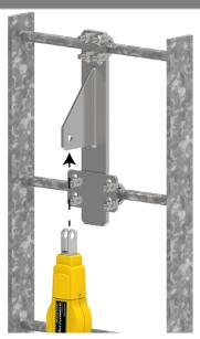
Secure the energy absorber and lifeline assembly with a carabiner and approved sling over the head and shoulder. Ascend the ladder using recognised twin hooking techniques ensuring the lifeline is safely managed by a second operative whilst unspooling at the bottom of the ladder.
