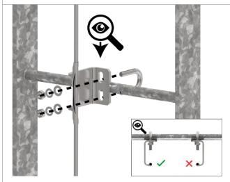
Ensure that the orientation of the cable guides suit the operation of the GTFA device and that the bracket is perpendicular to the rung. Loacte the cable into the helix slot of the cable guide.
