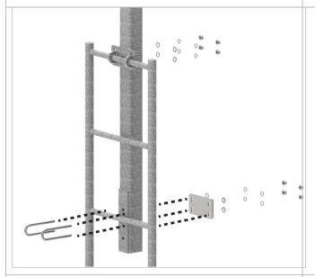
Secure the anchor bracket onto the top ladder rung with the shorter U-bolts and fixings from the extension post top anchor fixing kit. Hand tighten nuts to hold extension post in position.
