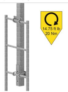
Evenly tighten the nuts to a torque of 14.75 ft lb (20 Nm).
