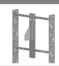
Locate the top anchor at the centre of the top two rungs as shown noting the orientation of the anchor fin and the four slots in the backing plate.
