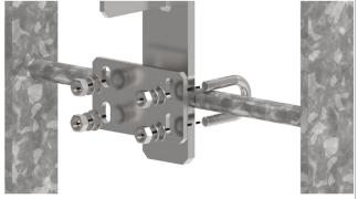
Attach the clamping plate in front of the anchor and secure into position with U-bolts and fixings from the top anchor fixing kit. Hand tighten nuts to hold anchor in position.
