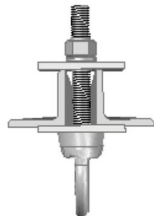
Figure 12 - Good Anchor Alignment
